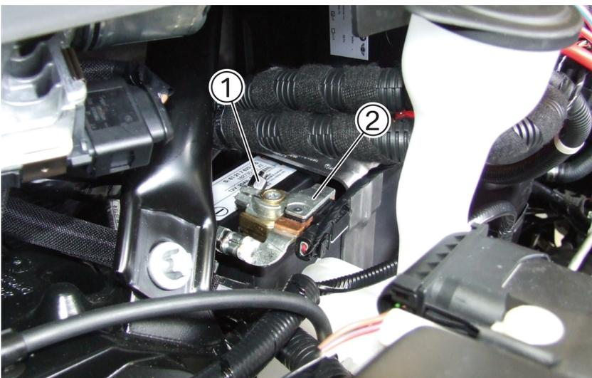
Slacken the nut (1) and pull off the battery earth lead (2) in the upwards direction. Cover negative battery terminal in order to rule out contact with battery earth lead.
