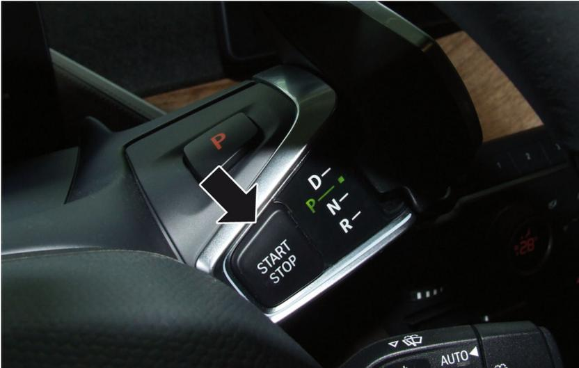
With the engine running or with the displays in the instrument cluster being activated, push button "START STOP" to switch off ignition.
