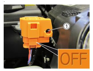
The high-voltage system is deactivated when bore hole (1) is completely free and the word "OFF" can be seen on the connector.
