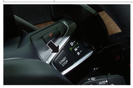
With the engine running or with the displays in the instrument cluster being activated, push button "START STOP" to switch off ignition.
