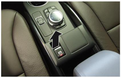
Pull the switch for the electrical Automatic Hold brake up.
