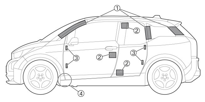
1. The areas mark the zones at which the roof can be cut off.
