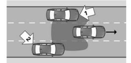
Radar sensors monitor the area behind and next to the vehicle when traveling faster than a minimum speed. The minimum speed is country-specific and displayed in the Active Blind Spot Detection menu.
