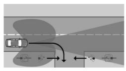
Sensors detect the traffic situation in their detection range when turning.
