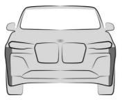
The radar sensors are located to the side in the front bumper.
