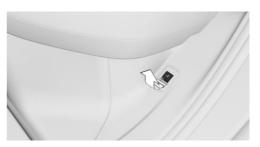
Pull the switch and fold the rear seat backrest. forward.
