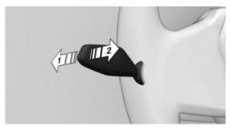
Press the turn signal lever forward, arrow 1, or pull the turn signal lever backward when the high beams are switched on, arrow 2.
