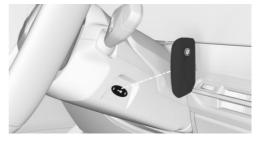
It is not possible to switch on drive readiness if the vehicle key has not been detected.
