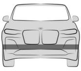
The ultrasonic sensors of the parking assistance systems are located in the area shown.
