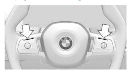
Depending on the equipment, the two LEDs above the keypads illuminate analog to the displays in the instrument cluster.
