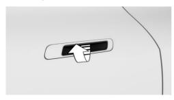
Press and hold the button in the recessed grip to unlock the vehicle and open the rear door.
