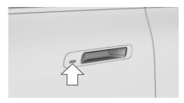
Touch the grooved surface on the external door handle of a closed vehicle door with your finger and hold it there without grasping the recessed grip.
