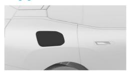
The charging socket cover is located in the rear on the right side of the vehicle.
