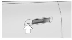
If you are carrying the remote control on your person, touch the grooved surface on the external door handle of a closed vehicle door with your finger for approx. 1 second without reaching into the recessed grip.
