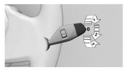
Turn the outer switch upward.
