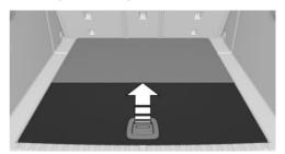
Pull on the handle and fold the cargo area floor forward.
