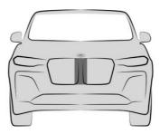
The radar sensor is located in the area shown.
