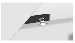
Pull the lever in the driver's door to unlock the driver's door.
