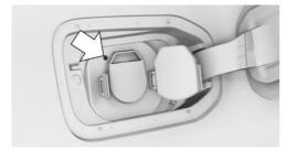
The charging status is indicated on the indicator light on the charging socket.
