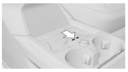
Two USB ports are located in the center console.
