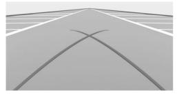
Turning circle lines can only be superimposed on the camera image together with pathway lines.
