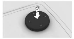
Slide in four directions to switch between menus, for example.
