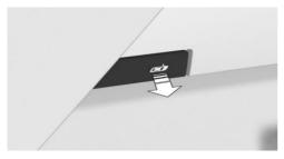
Pull the lever in the driver's door to unlock the driver's door.
