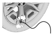
5. With the compressor switched off, insert the connector into the power socket in the vehicle interior.
