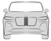
The front camera is located in the radiator grille.
