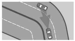
When you approach a curve the system may briefly report vehicles in the next lane due to the bend of the curve. If the system decelerates you may compensate for it by briefly accelerating. After releasing the accelerator pedal the system is reactivated and controls speed independently.
