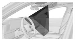
The camera in the headliner detects gestures that are carried out in the area of the center console at the height of the control display.
