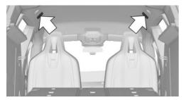
Insert each of the two top retaining pins of the cargo area partition net into the receptacles until they reach the stop, arrow 1, and push them forward. Make sure that the belt adjusters of the bottom hooks point to the front.
