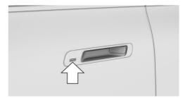
Touch the grooved surface on the external door handle of a closed front door with your finger and hold it there without grasping the recessed grip.
