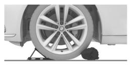
Place wheel chocks or other suitable objects in front and behind the wheel that is diagonal to the wheel to be changed.
