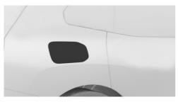
The charging socket cover is located in the rear on the right side of the vehicle.
