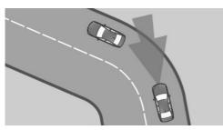
When the set speed is too high for a curve, the speed is reduced slightly. Because curves
