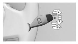
Turn the outer switch upward.
