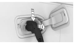
3. Detach the charging cable from the charging socket, arrow 2.
