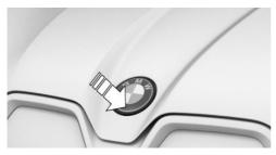
To open the container, press on the lower edge of the emblem on the hood. The lid opens when the vehicle is unlocked.
