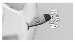
Turn the outer switch upward.
