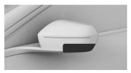
One exterior mirror camera is located at the bottom of each exterior mirror housing.
