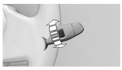
Turn the thumbwheel on the wiper lever.
