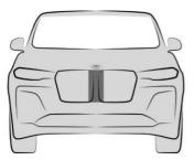
The front radar sensor is located in the radiator grille.
