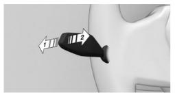
Press the turn signal lever forward, arrow 1, or pull the turn signal lever backward when the high beams are switched on, arrow 2.
