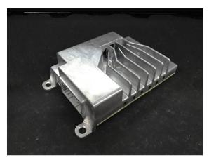
You will find the BMW amplifier in the trunk behind the right side panel. The amplifier is fixed with 3 screws
