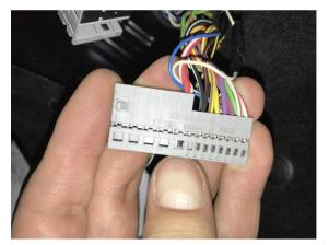
Take out the Black cable from the BMW connector (pin 2 (+)) and connect it to the blue plug on pin 17.
