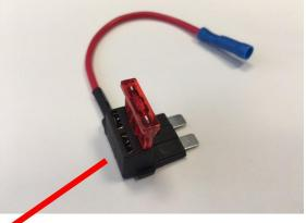
Remove the fuse 55 (5A) and insert it into the blank space in the fuse adapter.
