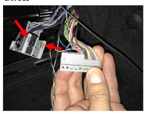
Slide the inlay out of the plug. To do this, press the latch (red arrow) outwards and pull out the inlay.
