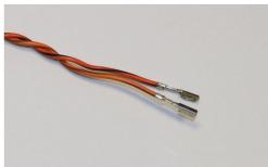
Connect the orange / black cable to the free space (Pin 18) where the white cable was plugged into the BMW control unit
