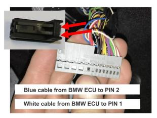
Disconnect the Blue cable (Can Low) from pin 19 and pin it on the supplied black plug on pin 2.
