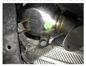
On the BMW i8, a speaker actuator is already installed under the vehicle on the left.
