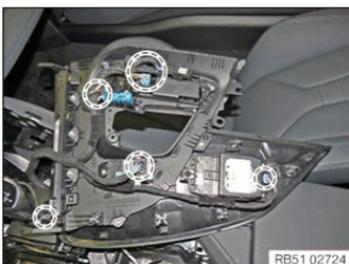
Disconnect the plug connections.
