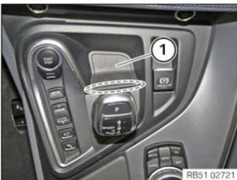
Lever out the cover (1) at the mark using the special tool 64 1 020.
