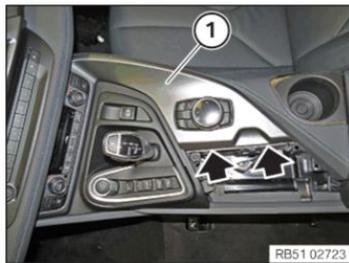
Lever out the center console trim (1) at the marked positions.
