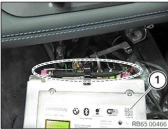
Unlock and disconnect all connectors in marked area.
